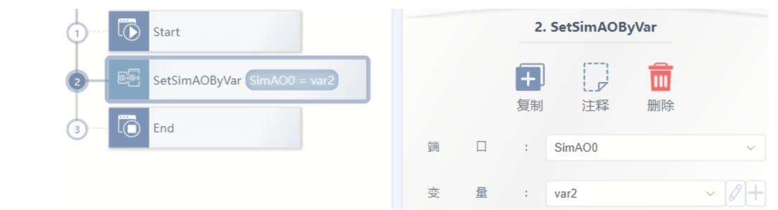
The diagram shows a sequence of three steps: 1. Start, 2. SetSimAOByVar (SimAO0 = var2), and 3. End. The configuration interface for '2. SetSimAOByVar' includes buttons for '复制' (Copy), '注释' (Comment), and '删除' (Delete). It features a dropdown menu for '端口' (Port) set to 'SimAO0' and a dropdown for '变量' (Variable) set to 'var2'.
